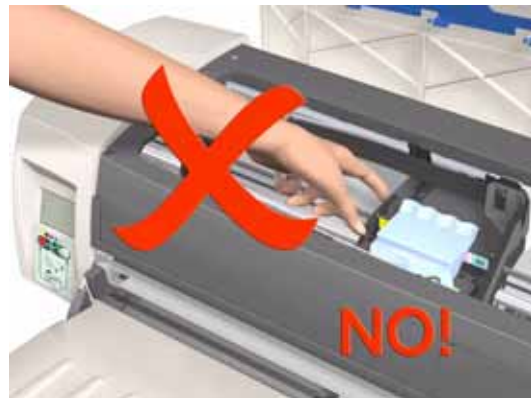
Incorrect: never move using Carriage Assembly.
