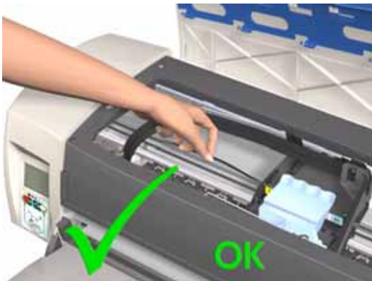
Correct: move using the belt.
